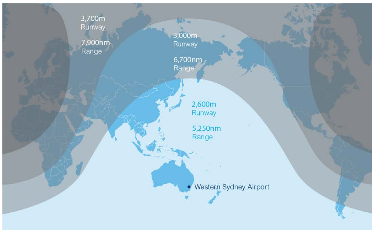
Figure 5–7 – B777-300ER range with 100 per cent passenger load
