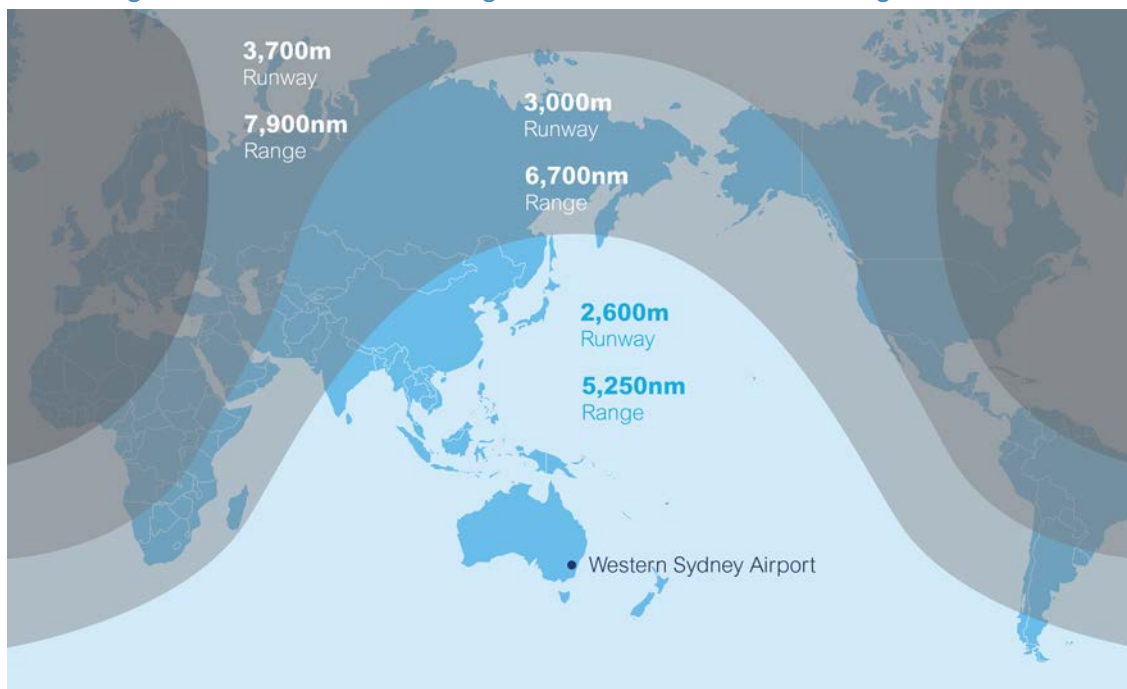
Figure 7: Boeing 777-300ER indicative range with maximum take-off weight
