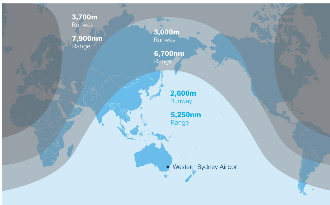
Figure 7: Boeing 777-300ER indicative range with maximum take-off weight
