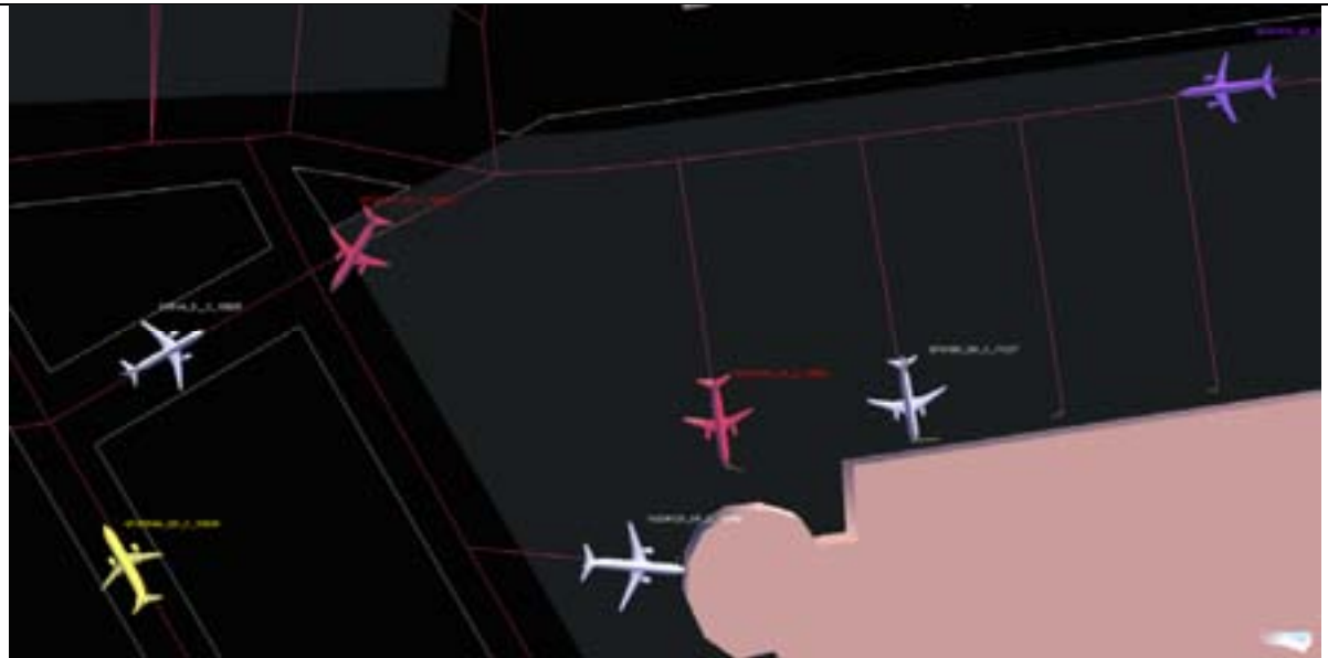
Figure 9.13 - Alleyway Interference between Departing and Arriving Aircraft
