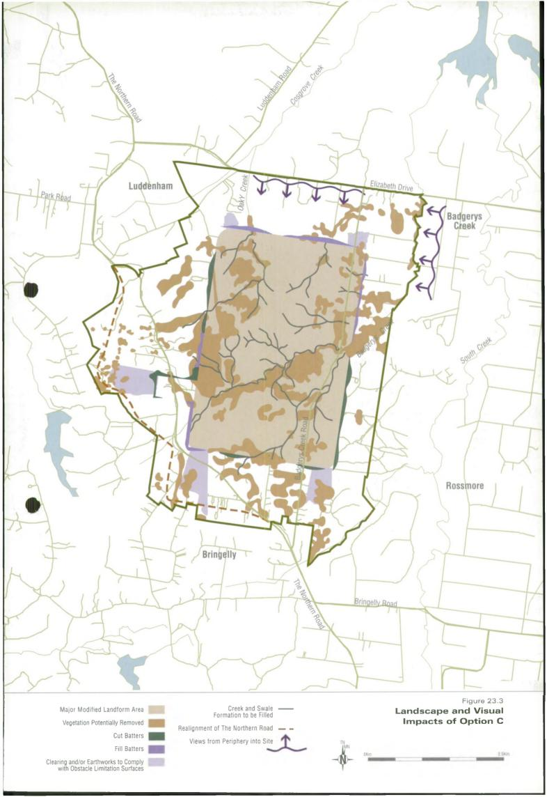
runways, taxiways, terminal and apron reserve areas. The platform would be established essentially by filling the upstream section of Badgerys Creek, cutting the elevated areas south and north of the creek, and filling the lower northern areas of the site. Unlike Options A and B most of the western ridgeline would remain; only a small section would be cut. Impacts on vegetation would be similar in extent to those for Option B.
