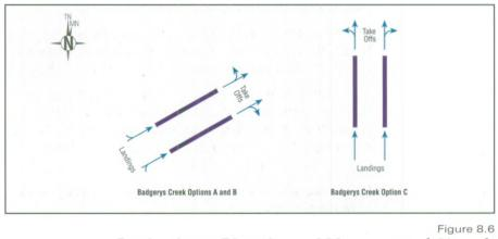
**Predominant Directions of Movement of Aircraft** for Airport Operation 1 Note: Cross wind runway used only when required because of meteorological conditions
