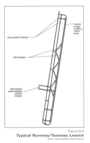
The cross wind runway would be linked by rapid exit and other taxiways to two full length parallel taxiways designed to accommodate Code F aircraft for the section between the parallel runway system, and Code E outside the parallel runways.
